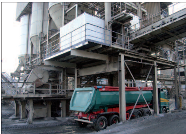
HAYER CPA CONTAINER analysing a slag-sand mixture
