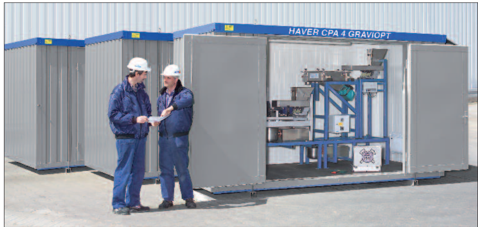
HAYER CPA CONTAINERS with Photo-Optical Particle Size Analysers as "Plug and Play" solution
