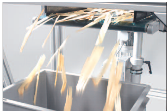
HAVER CPA 4 CONVEYOR analysing size and shape of wood chips
