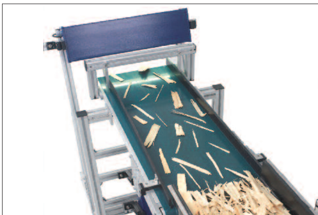
HAVER CPA 4 CONVEYOR, alignment and separation of longish samples on the conveyor
