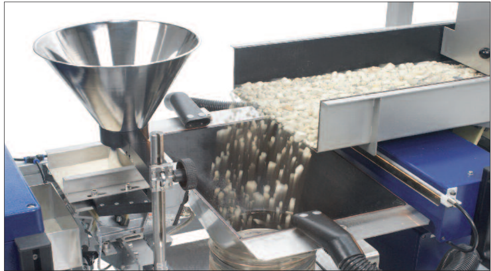
HAYER CPA 4-2 measuring gravel and sand in two measuring ranges
