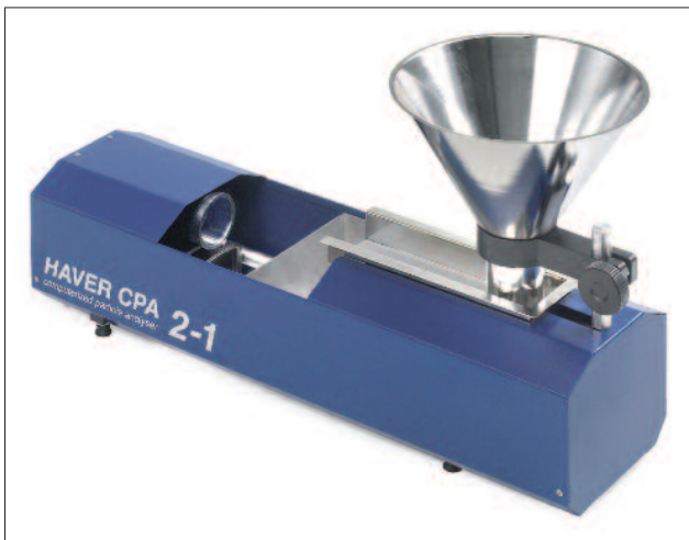
HAVER CPA 2-1, laboratory unit for particle size and shape analysis in the measuring range from 34 µm up to 25 mm
